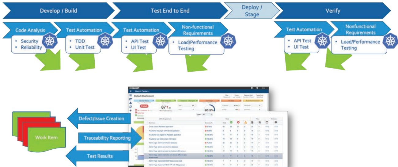
Figure 9-4: Parasoft provides bidirectional traceability from work items to test cases and test results, displaying traceability reports with Parasoft DTP and reporting results back to the requirements management system.
