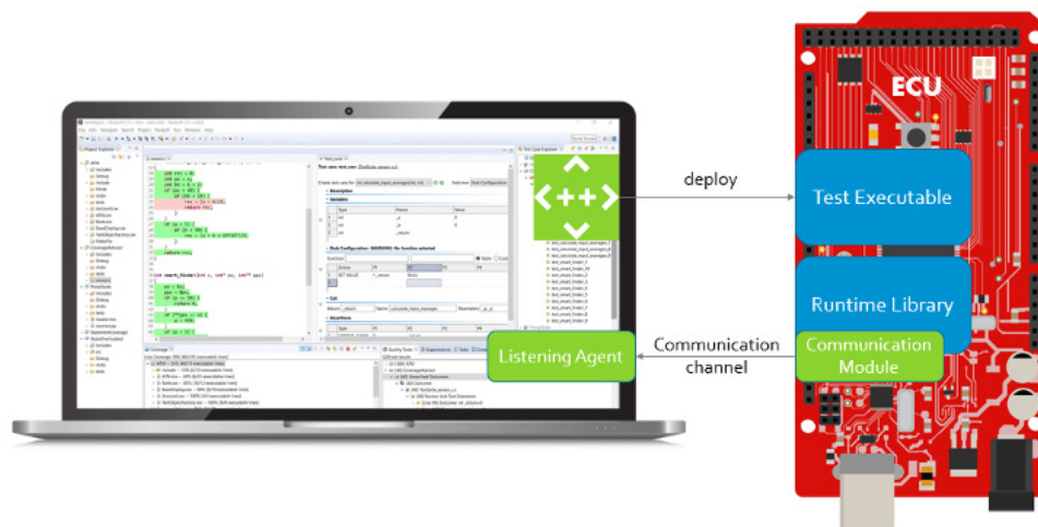
Figure 4: A high-level view of deploying, executing, and observing tests from host to target.
