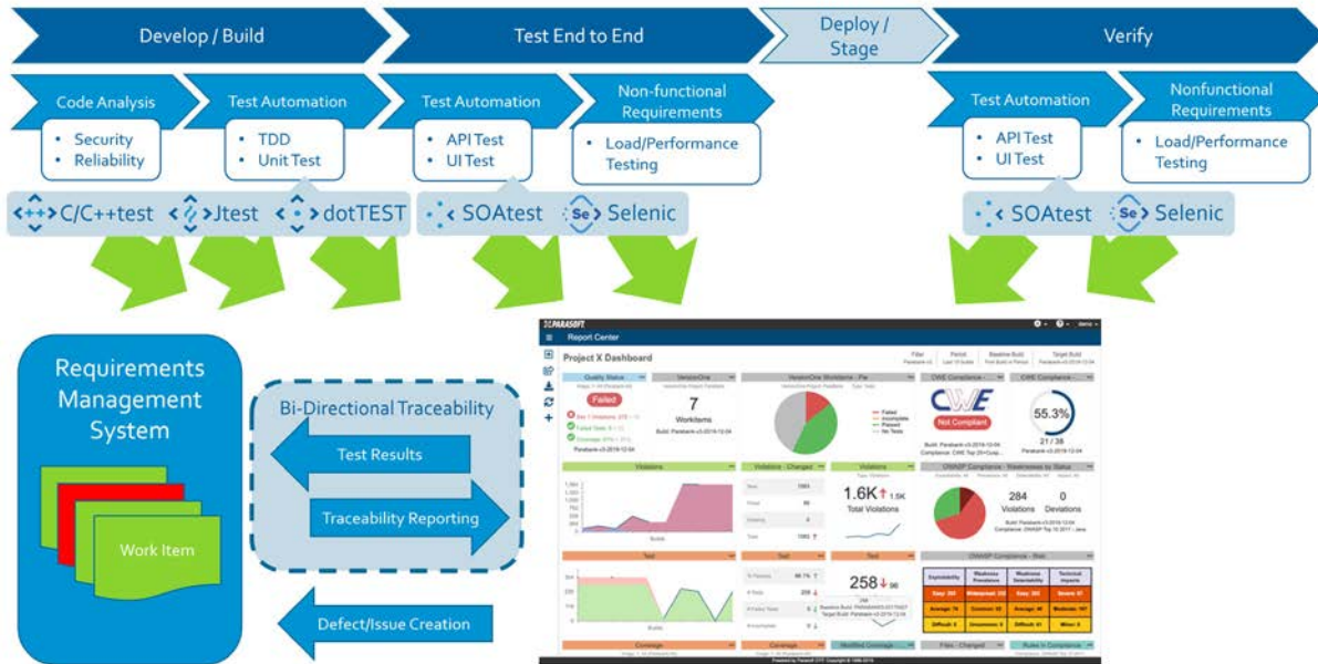
Figure 9-4: Parasoft provides bidirectional traceability from work items to test cases and test results, displaying traceability reports with Parasoft DTP and reporting results back to the requirements management system.
