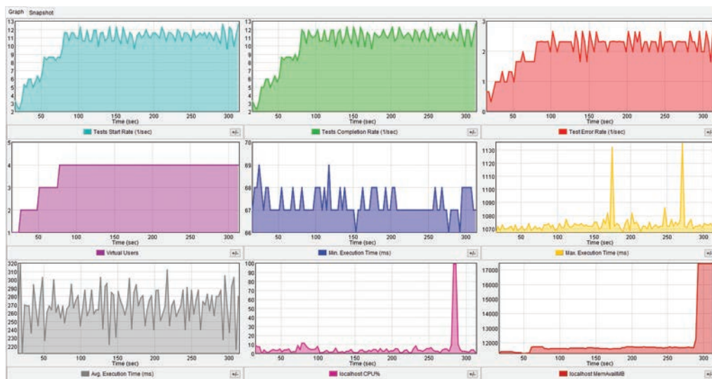
Figure 2: Progress graphs of a performance testing tool executing a performance test.
