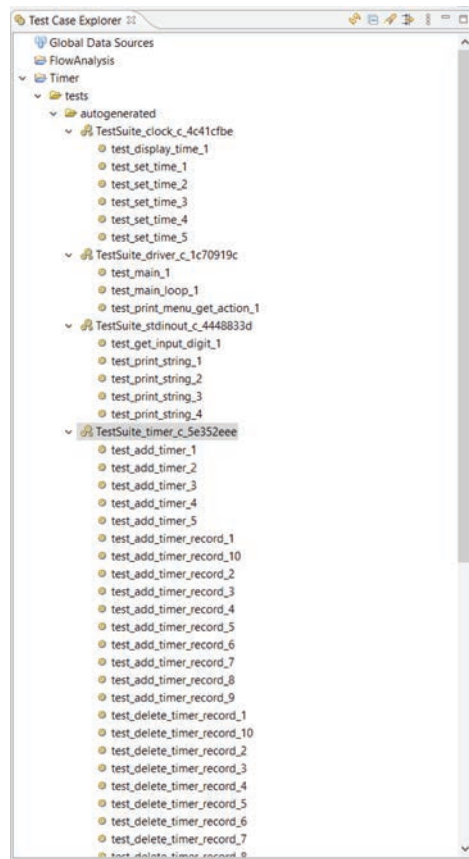
Figure 2: Example of an automated test case generation. In this case, one test suite per function.
